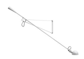
Wall lamp providing direct light. Painted steel adjustable arm and reflector. Chrome-plated brass reflector support. Cast iron tapered counterweight. Painted steel wall fixture.
