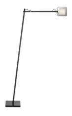
Floor lamp. Head in pressofused aluminium, diffuser in PC. Power pack on plug, base cover in injection printed PC, counterweight in iron cut and painted by means of a cataphoresic process. Directionable head. Three-step ON/OFF switch with Soft Touch technology. Base separated from the lamp body with safety locking pin.
