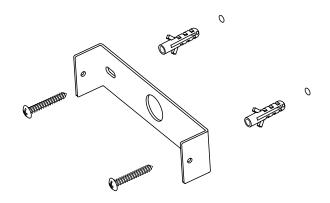
4. Attach the mounting cup to wall bracket by fastening the screws
