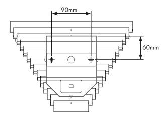
1.Remove the wall bracket by unfastening the screws. Be careful not to damage the shade.
