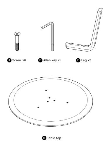
Fasten the legs **©** to the table top **D** with the screws **A**, using the Allen key **B**. Start by loosely tightening all the screws before tightening them all completely.
