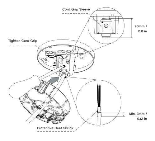
It is advised that any wire exposed with just a single basic layer of insulation is covered with the protective heat shrink provided. (Two sleeves for the basic insulated wire and one sleeve for covering the opening of the source cable).
