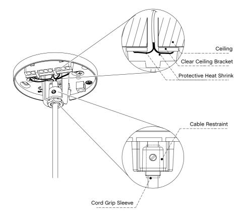
If utilising the mouse hole cable exit, please note the internal cable restraint and integrated cable clamp. The cable clamp tab can be removed and cut to length to suit the cable thickness used, if this is larger than what is already provided.
