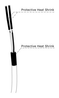
A heat gun can be used to shrink and fix this protective insulation in place, as shown below.
