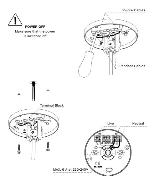
The terminal blocks of the clear ceiling bracket are integrated into a junction box with a loop-in feature. This can be utilised in a number of different ways to optimise the wiring of electrical fittings used in your environment, either for single light fixtures and switches, multiple light fixtures to a single switch, or even lamps and ceiling fans connected to a single switch.
