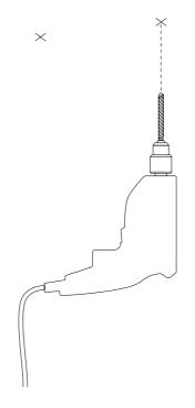
Trim the cable to the desired length, leaving 35 mm / 1.4 in of basic single insulation exposed for wiring.
