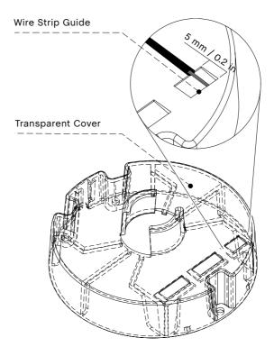
It is advised that any wire exposed with just a single basic layer of insulation is covered with the protective heat shrink provided. (Two sleeves for the basic insulated wire and one sleeve for covering the opening of the pendant cable).
