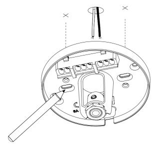
Drill holes and insert wall plugs. Ensure you use the correct type of drill and wall plug / anchor for the material you are drilling into.
