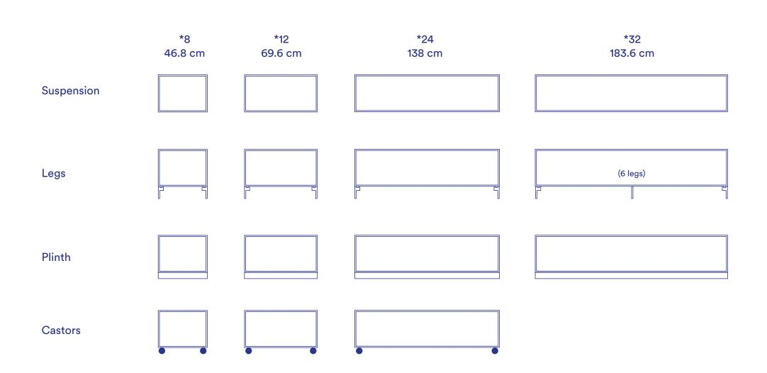
Selected basic assortment of system units to configure from. Choose depth (30 & 38 cm), position and colours. Predefined slot for cable pass in partitions  $\leftrightarrow$
