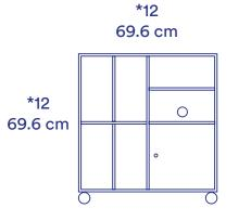
SPIN II Depth: 46.8 cm Incl. (KABELD) Follows colour of module Positions: Castor CR70 black, legs, wall-mounted
