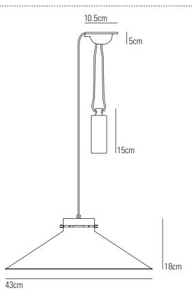
Cable length may be shortened upon installation. This will reduce both maximum & minimum drop and reduce the range of movement.
